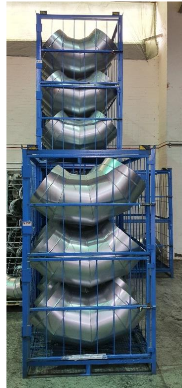
Figure 2 Illustration of a steel stillage that carries the fittings.
