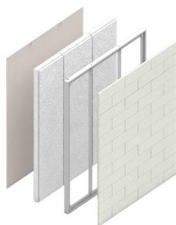
Figure 1: Exploded view of Nexii panel
